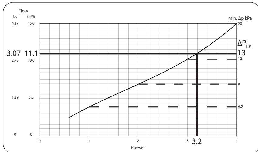
The selected OPTIMA Compact EP DN50 LF requires  $\Delta P_{EP} = 13$  kPa of differential pressure and should be set to position 3.2 to provide the sizing flow.
