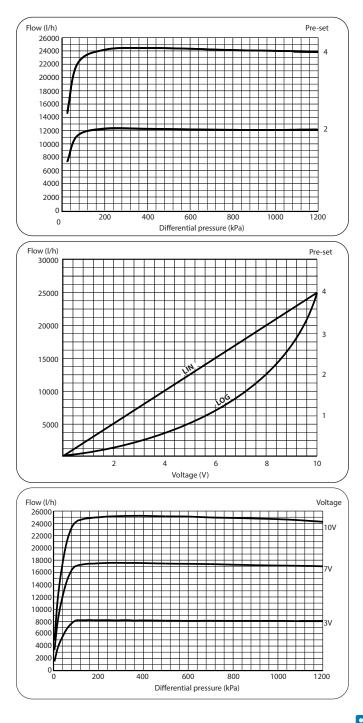
Flow rate vs. Voltage
