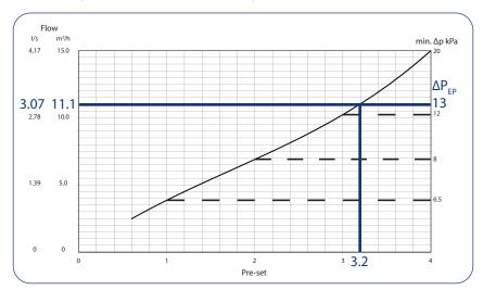
The selected Frese OPTIMA Compact EP DN50 LF requires  $\Delta P_{EP} = 13$  kPa of differential pressure and should be set to position 3.2 to provide the sizing flow.
